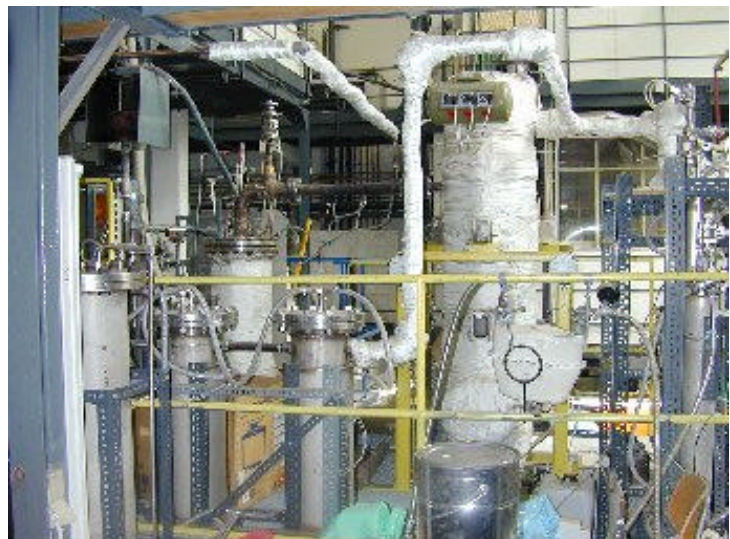
Figure 5 70 mm Entrained-flow Gasifier at EBI
